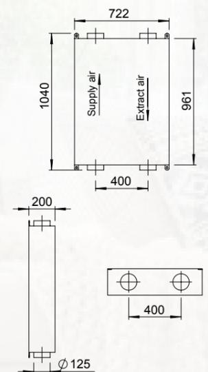
Standard 4x 125mm Ports are placed at the top and bottom of the item to give straight through duct connections. Compact design with easy installation and maintenance. Please see above image for the individual dimensions. Unit supplied with two inspection covers, one on each side enabling the unit to be left or right handed.
